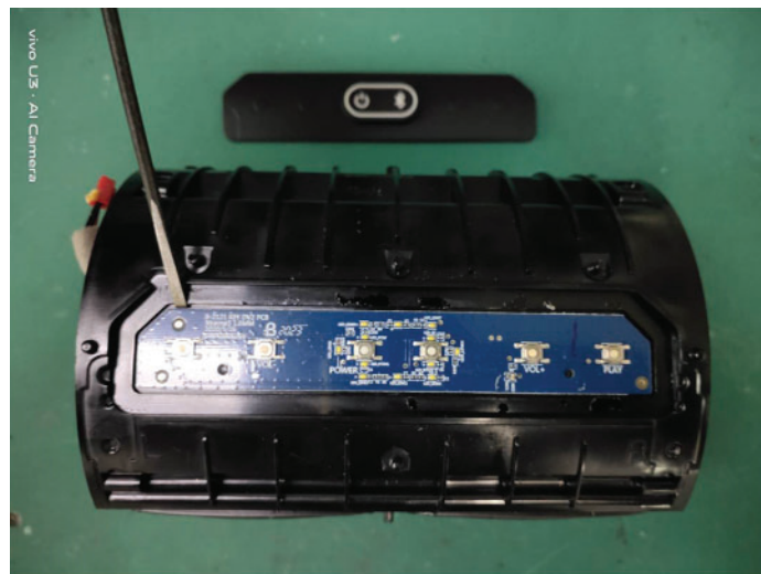
11. Use a pry knife to pry and open the buttons board.
