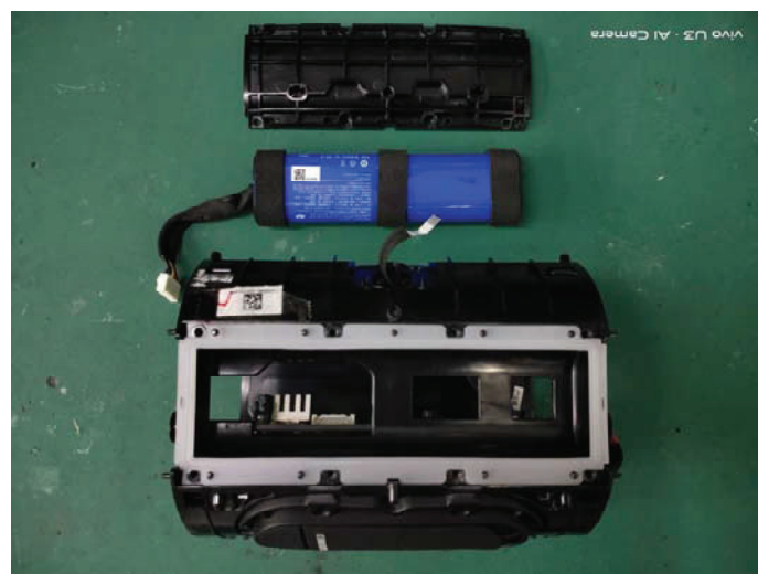
15. Loosen 8 screws, remove the battery cover and battery.
