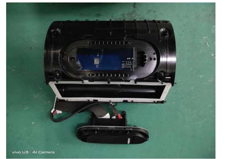
16. Loosen 6 screws, remove the I/O stents and jack board.
