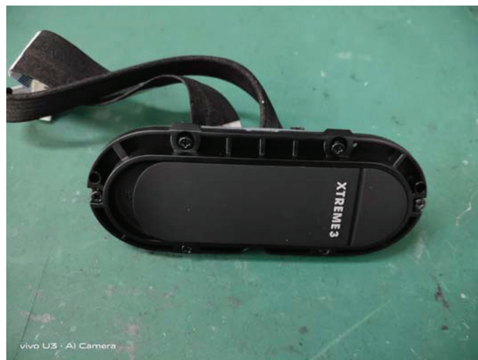
17. Pull out the the I/O cover by hand.
