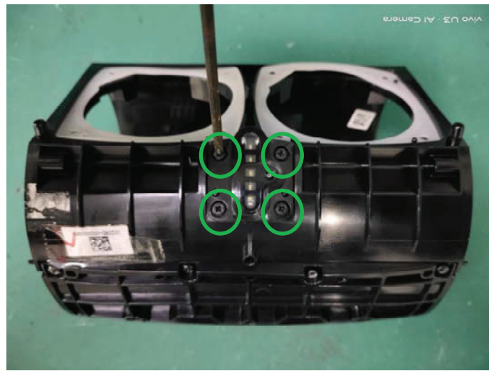
15. Loosen 8 screws, remove the battery cover and battery.
