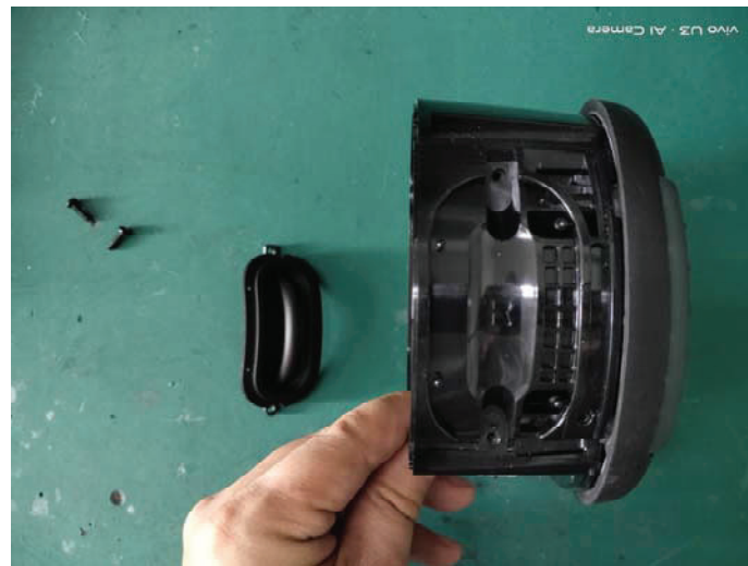
9. Loosen 2 screws, remove the right hook bridge hook cover.
