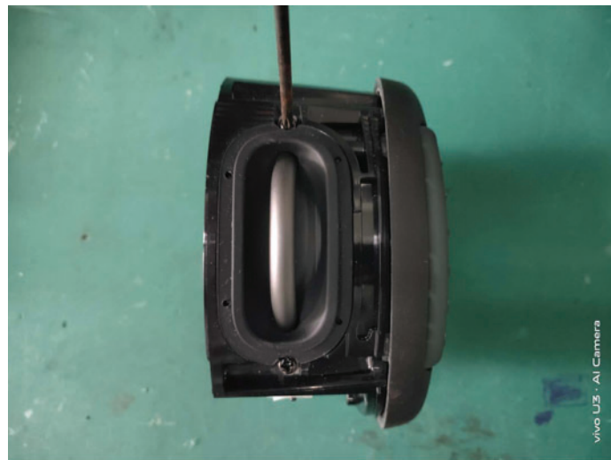
11. Use a pry knife to pry and open the buttons board.
