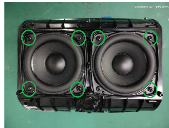
12. Loosen 8 screws, remove the 2 woofers.
