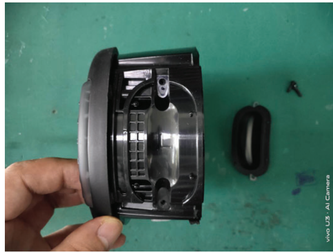
9. Loosen 2 screws, remove the right hook bridge hook cover.
