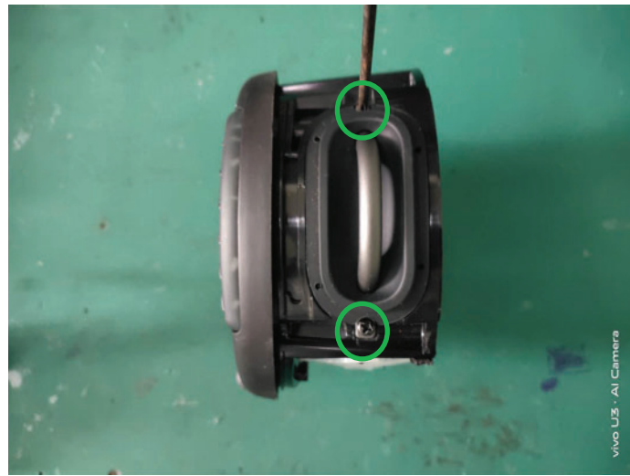
9. Loosen 2 screws, remove the right hook bridge hook cover.
