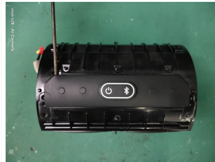
12. Loosen 8 screws, remove the 2 woofers.
